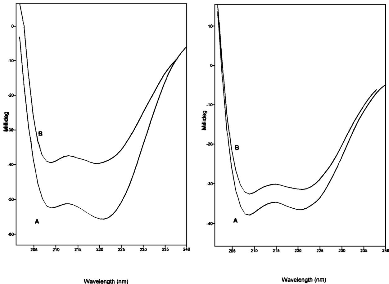
Fig. 4. Circular dichroism spectra of HtrX (left panel) and HtrXI (right panel) in the presence of 3.6 M NaCl (A) and 3.6 M KCl (B). Sample conditions are as described in Fig. 1.
