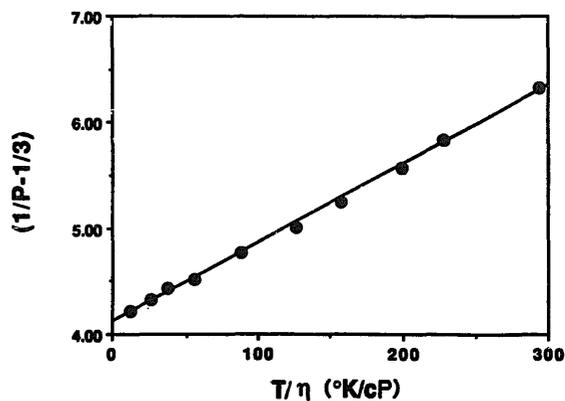
Fig. 3. Perrin plot for HRP(desFe) at 22°C; viscosity was varied by sucrose addition. Excitation wavelength was 514 nm; emission was observed through a Corion LL 600 cuton filter which passed  $\lambda > 600$  nm.
