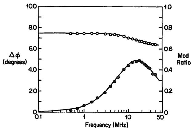
Fig. 4. Differential phase (●) and modulation (○) data for HRP(desFe); experimental conditions the same as in Fig. 3. Solid curves correspond to values obtained for the best-fit analysis of phase and modulation data;  $\rho_1 = 86$  ns,  $\rho_2 = 12$  ns,  $a_1 = 0.163$ ,  $a_2 = 0.005$ .
