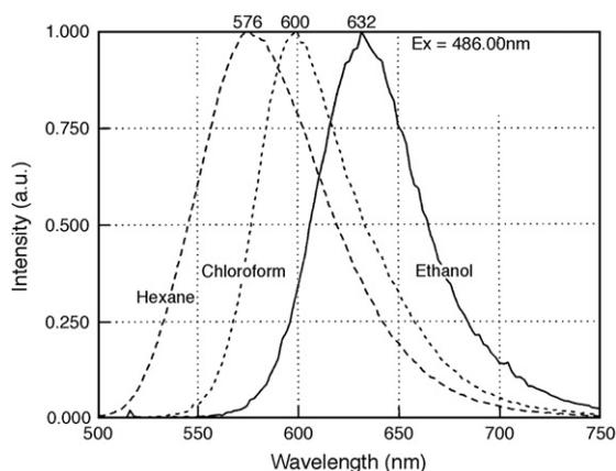
Fig. 1. Technical emission spectra for Nile Red in various solvents. The emission spectra normalized at their maxima to emphasize the wavelength shift. Dielectric constants: hexane, 1.89 at 20 °C; chloroform, 4.8 at 20 °C; ethanol, 24.3 at 25 °C.
