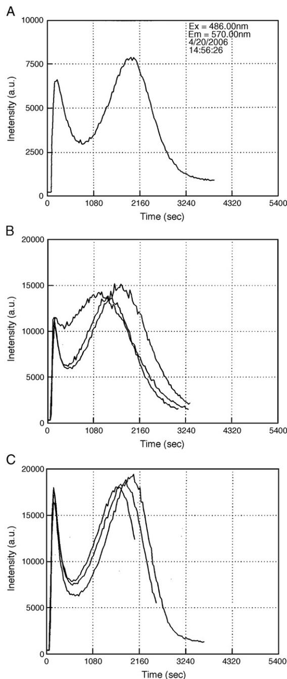
Fig. 2. Typical time-varying intensity emission profile of Nile Red excited at 480 nm and recorded at 570 nm after addition to a solution of live *Nannochloropsis* sp. cells (A). Multiple responses of live *Nannochloropsis* sp. cells at an OD<sub>720</sub> of 0.1 (B) and live *Tetraselmis* sp. cells at an OD<sub>720</sub> of 0.1 (C).
