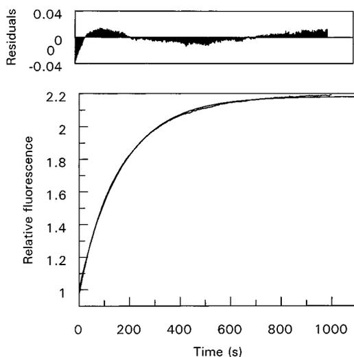
FIGURE 8: Stopped-flow record of the release of  $\text{P}_i$  during a single turnover of GTP by dynamin. One syringe contained  $5 \mu\text{M}$  dynamin, and the other contained  $2.5 \mu\text{M}$  GTP. Both syringes contained  $13 \mu\text{M}$  coumarin-labeled phosphate binding protein. The solid line is the best fit to a single exponential with a rate constant of  $0.0061 \text{ s}^{-1}$ .
