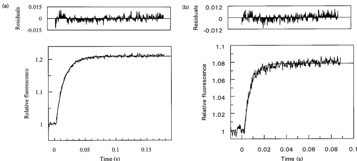
FIGURE 2: Stopped-flow fluorescence record of the binding of mantdGTP and mantdGDP to dynamin. One syringe contained  $1 \mu\text{M}$  dynamin, and the other syringe contained (a)  $30 \mu\text{M}$  mantdGTP and (b)  $30 \mu\text{M}$  mantdGDP. The solid lines are best fits to the data to a single exponential giving rate constants of (a)  $75$  and (b)  $171 \text{ s}^{-1}$ . The data are the averages of four reactions.
