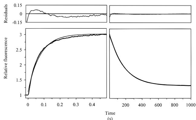
FIGURE 6: Stopped-flow fluorescence record of a single turnover of mantdGTP by dynamain. One syringe contained  $5 \mu\text{M}$  dynamain, and the other syringe contained  $2.5 \mu\text{M}$  mantdGTP. The time course was followed over  $0.5 \text{ s}$  (left panel) and  $1000 \text{ s}$  (right panel). A fit of the slow process to a single exponential gives a rate constant of  $0.0056 \text{ s}^{-1}$ .
